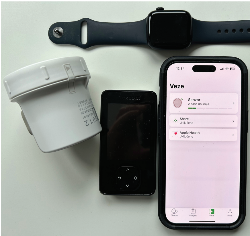
Figure 1: Dexcom One+ is combined with a device accompanying the sensor, a smartphone application, and a smartwatch
